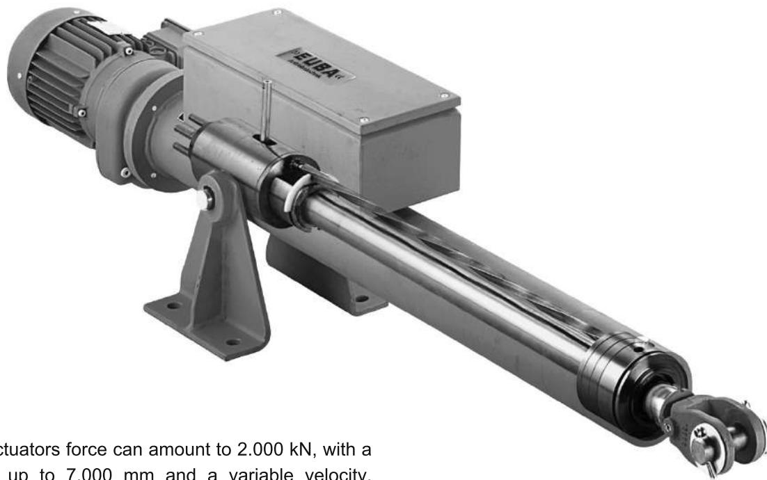
The actuators force can amount to 2.000 kN, with a stroke up to 7.000 mm and a variable velocity. Normally our actuators are manufactured with a hard chromium plated pushrod (special requests such as a ceramic plated pushrod can be considered). Commercial motor-gear combinations (A.C., D.C., et al.), which are connected to the actuator by a DIN IEC flange, are used. Rotary actuators, which are able to do complete revolutions, can also be flanged.
