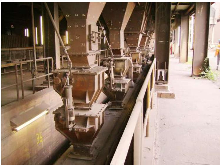
Double Cone Lock Sinter Plant
